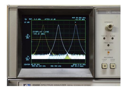
The NewScope-8 Color LCD replacement Kit is designed to replace the monochrome CRT in the HP® 85662A spectrum analyzer display. The Kit supports 6.4" or 6.5" TFT color LCD with VGA (640 x 480) or XGA (1024 x 768) resolutions.
